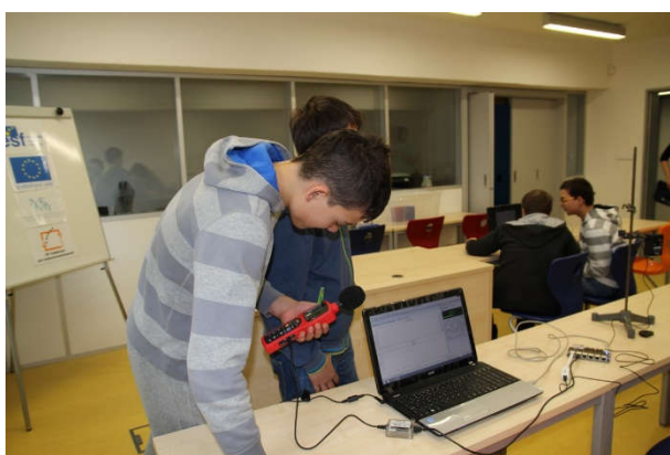
Fig. 2: Measuring of noise by the sound level meter and the EdLab measuring interface
