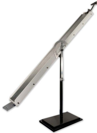
Fig. 1: Newly designed school inclining tribometer
