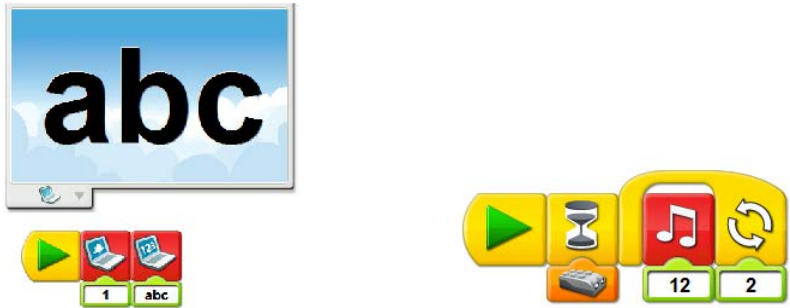
Fig. 2: (a – on the left) A picture 1 and the text “abc” are shown on the virtual display. (b – on the right) The program is waiting until it sees something (wait until), then it emits a whistling sound twice (the for loop).
