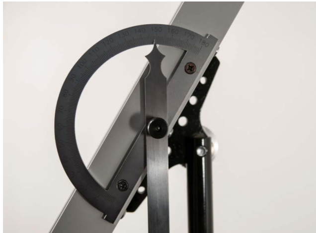
Fig. 2: Universal protractor attached to the inclining tribometer
