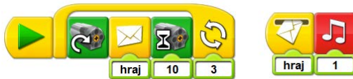
Fig. 1: showing the simulation of the play procedure (on the right), when together with three repeated moves of the motor, there is a parallel sound.
